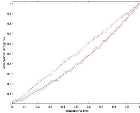
**Fig. 2.** Black and red curves correspond to the haptic stimulus without and with the vibrotactile mode respectively. Dash-dot curves refer to the linear signal (quasi-periodic state, herefore red curve has a constant frequency), while curves with solid lines correspond to the non-linear signal (chaos state, herefore red curve has an exponential increase of its frequency).
