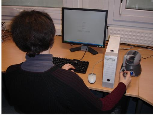
**Fig. 3.** Experimental setup: the user holds the haptic arm with the dominant hand and interacts with the graphic interface with the non-dominant hand (keyboard). The box prevents the visual observation of haptic stimuli (i.e., movements and oscillations)
