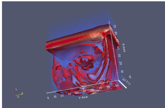
**Figure 2.** Lagrangian Coherent Structures in the 3D numerical cavity flow. Only the central third of the spanwise direction is represented.
