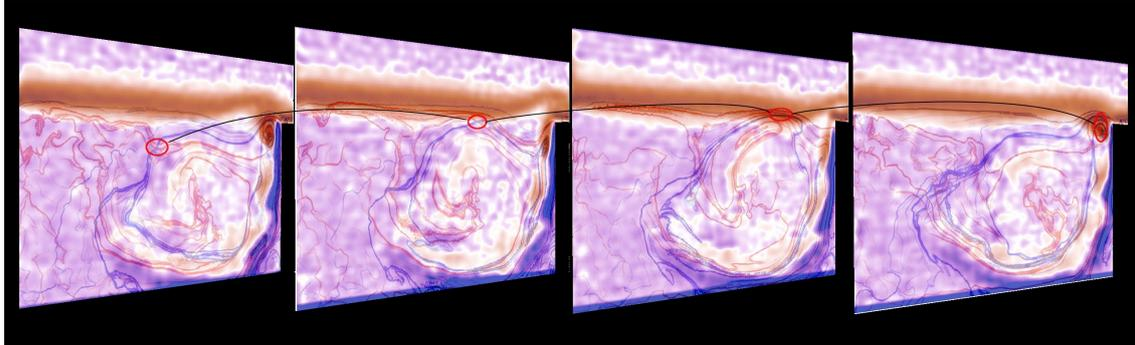
**Figure 1.** Tracking of an hyperbolic point in the experimental 2D PIV dataset. Red and blue lines represent finite-time attractive and repulsive LCS while the background field is the vorticity field.
